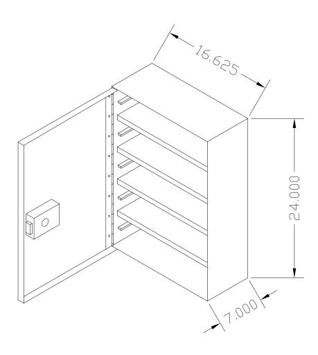
CONSTRUCTED WITH 10 Ga. STEEL DOOR IS HUNG ON A HEAVY DUTY CONTINUOUS HINGE AND LOCKED WITH A DETENTION DEADLOCK.
